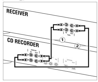
Use the audio cables supplied. Connect the red plugs to the R sockets, and the white plugs to the L sockets.
